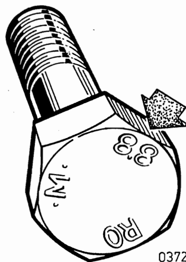
Fig 2 Bolt grade marking
